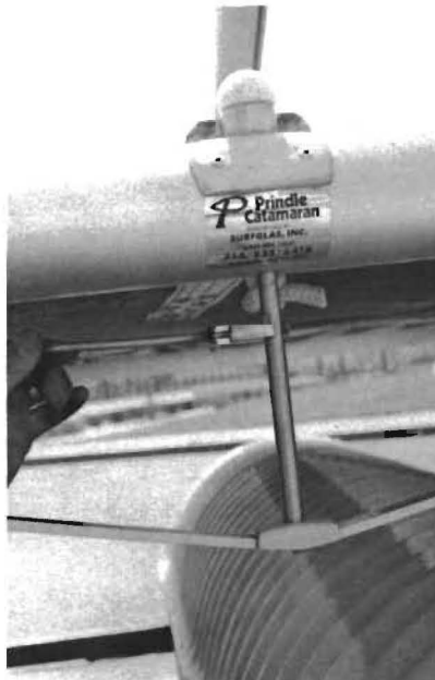
Loosen screw at bottom of striker rod.
