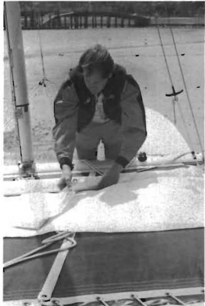
Fold the jib in half and start rolling from the middle.
