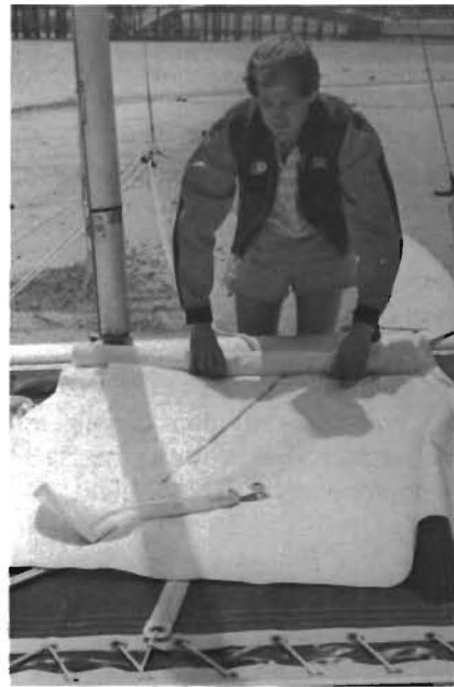
Fold the jib in half and start rolling from the middle.
