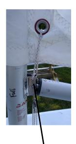
The fixed short line is attached permanently to the port side of the goose neck. It is about one foot long and has a sister clip attached at its end....
