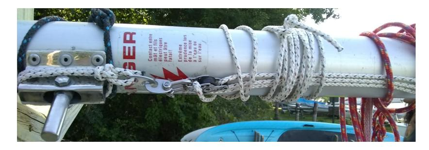
Wrap the short line of the downhaul around the gooseneck as shown. Join sister clips, tighten a bit, then coil or wrap the downhaul line around the mast.
