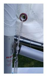
... Feed it through the cringle, sister clip first, and pull downwards on starboard to connect to the matching sister clip on the downhaul assembly, on the right ->
