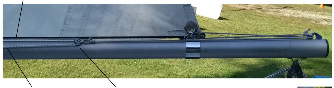
The loose end of outhaul line exits this little block, runs back to the mast on the port side of the boom.
