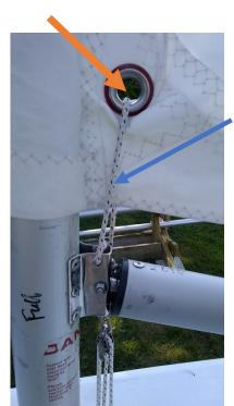
The fixed short line is attached permanently to the port side of the goose neck.
