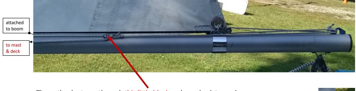
The outhaul returns through this little block and runs back towards the mast on the port side of the boom, where....
