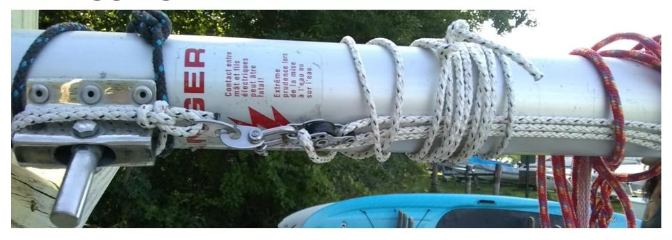
**Downhaul / Cunningham:** Wrap the short line of the downhaul around the gooseneck as shown. Join sister clips, tighten the downhaul line bit, then coil or wrap the downhaul line around the mast.
